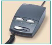
The GN 8000 Series Multi-Purpose Amplifier works with most phone systems with a modular handset connector. It features a built-in headset stand with an on-line indicator option that signals when the headset is in use.
